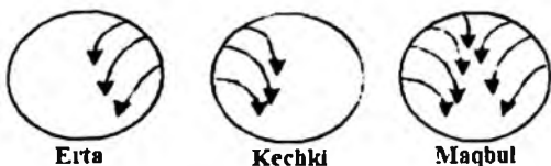
117 – rasm. Klinkerning rekuperatorda taqsimlanish sxemasi
