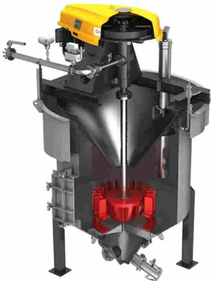
118-rasm. Tezkor (flesh) flotatsiya mashinasining qirqimda ko‘rinishi
