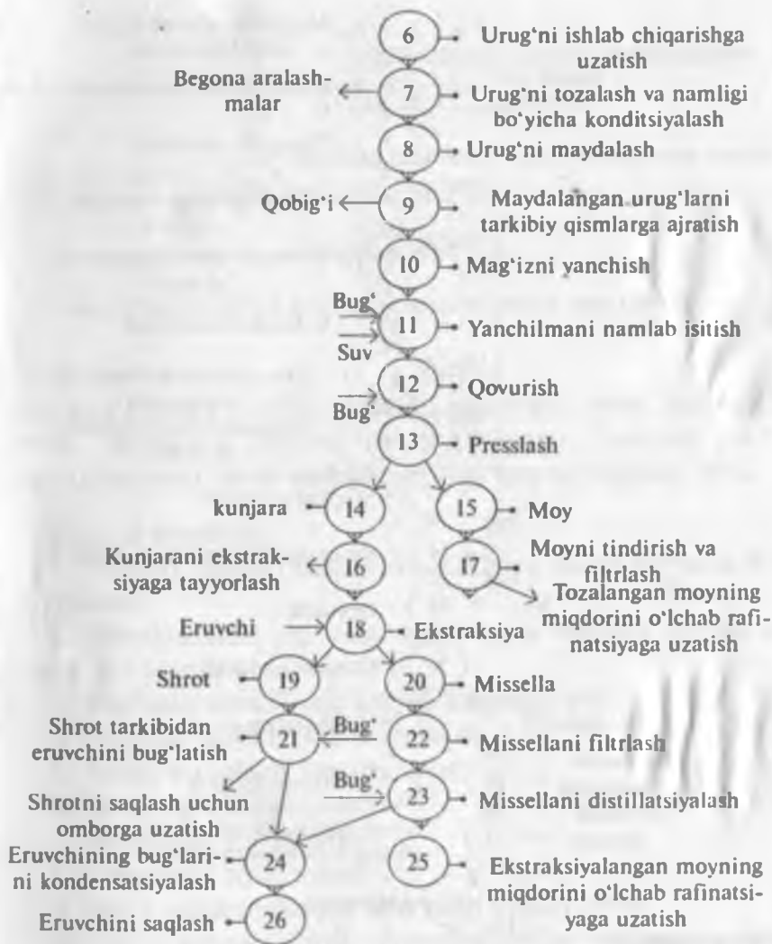
2-rasm. Moyli xomashyolardan forpress-ekstraksiya usulida moy olish.
