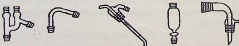
9-rasm. Shlifli nasadkalar, tomizgich voronkalar va shlifli alonj.
