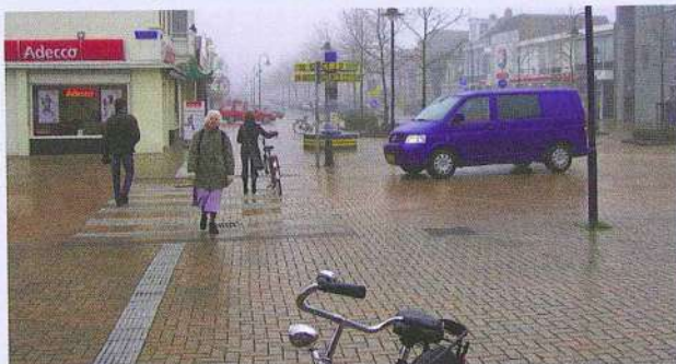
Pedestrians, bicycles, and cars all share this intersection in Drachten without the need for traffic lights or road signs.
