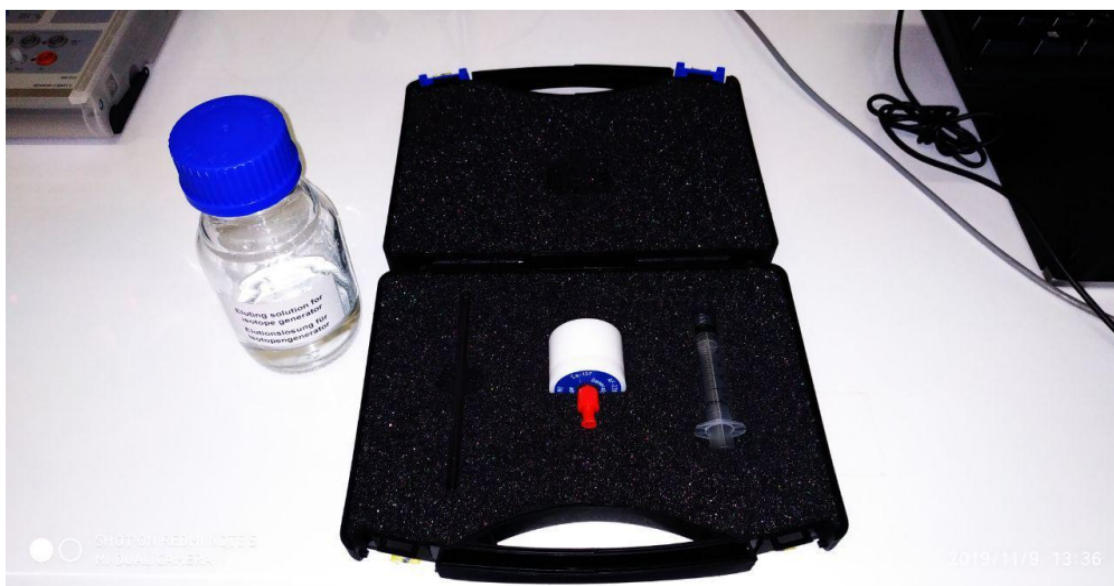
4-rasm. Ba – 137 m ni Cs/Ba – 137 m izotop generatoridan yuvib olish.
