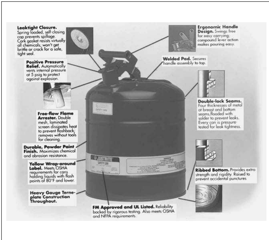
Figure 8-4. Example of flammable liquid safety can with illustrated safety features.
