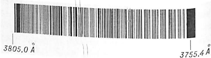
1-rasm. Azot molekulasining spektral polosasining spektral chiziqdagi ajralishi
