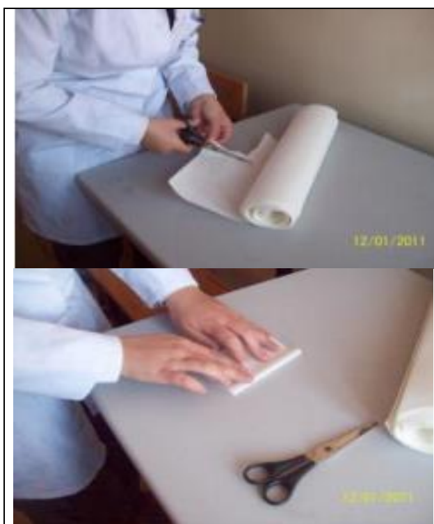
Rasm. 52. Tekis filtrni tayyorlash.
