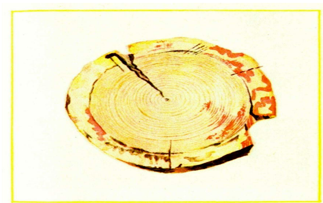
1-rasm. Yog'ochning yorilishi.
