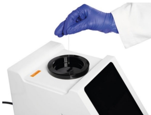
4-rasm. Salomas qattiqligini Mettler Toledo laboratoriya asbobida aniqlash jarayoni
