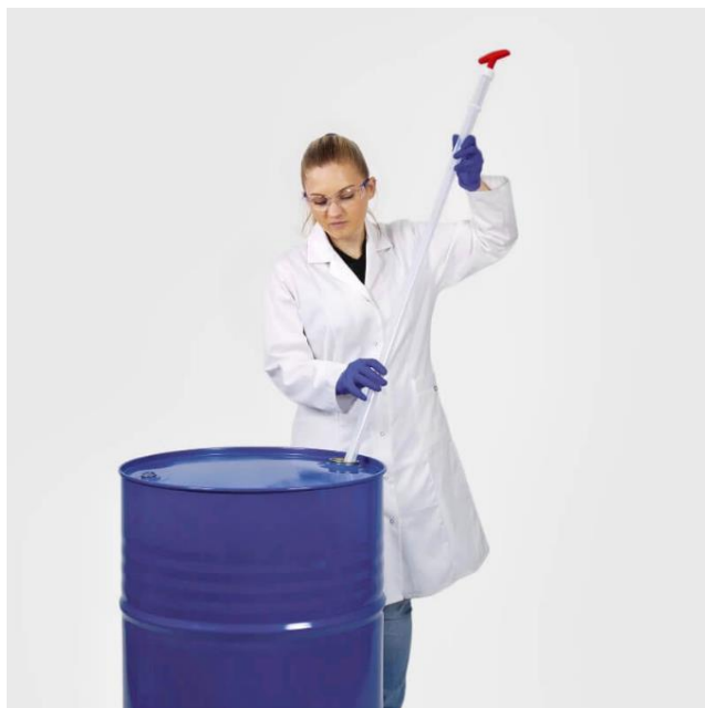
Rasm 3. Metall idishdan glitserin namunasini olish jarayoni
