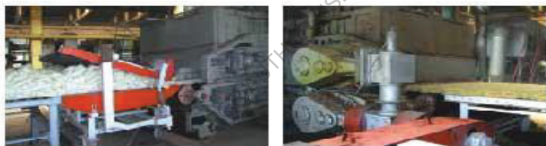
27- rasm. Mineral korpaga issiqlik ishlovini berish.
