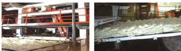
26- rasm. Mineral tolali ko'rpa hosil qilish.
