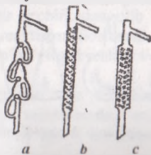
5-rasm. Deflegmatorlar: a-sharikli; b-archasimon; c-nusadkall
