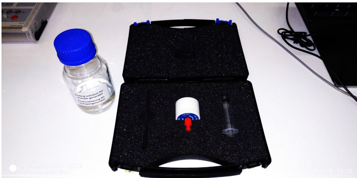
4-rasm. Ba – 137 m ni Cs/Ba – 137 m izotop generatoridan yuvib olish.
