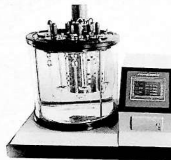
2.2-rasm. Neft mahsulotlarining kinematik yopishqoqligini VISCOMETER ASTM D 445 qurilmasida tekshirgich
