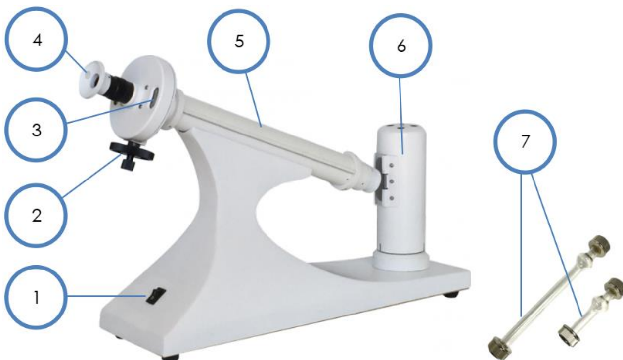
3.3-rasm. Polyarimetr. 1 - yoqish tugmasi; 2 - analizatorning burish vinti; 3 - asbob shkalasi; 4 - ko'rish trubkasini fokuslash muftasi; 5 - kyuvetalar uchun kamera; 6 - yorug'lik manbai; 7 - kyuvetalar.
