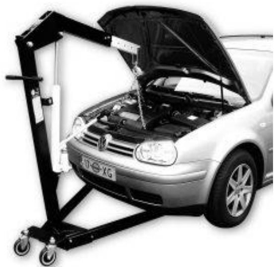
6.13b-rasm. Buklanuvchan xarakatlanuvchi kran (rusumi-5.1310, yuk ko'tarish qobiliyati 250-500-750-1000 kg., ilib olish balandligi-min 10-100-190-280 mm, max 2030-1955-1880-1805 mm, ko'tarish uzunligi 1100-1010-920-830 mm., tashqi o'lchamlari 1260x980x1400 mm, massasi 75 kg).
