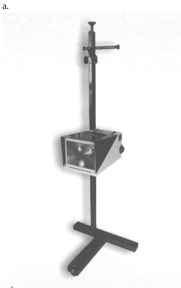
6.37-rasm. Avtomobil farala-rining parametrlarini diagnos-tikalash uchun IPF-01 jixozi (a) va tekshirish jarayoni (b).
