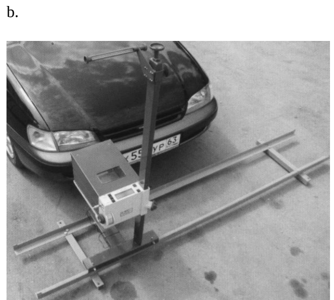
6.37-rasm. Avtomobil farala-rining parametrlarini diagnos-tikalash uchun IPF-01 jixozi (a) va tekshirish jarayoni (b).
