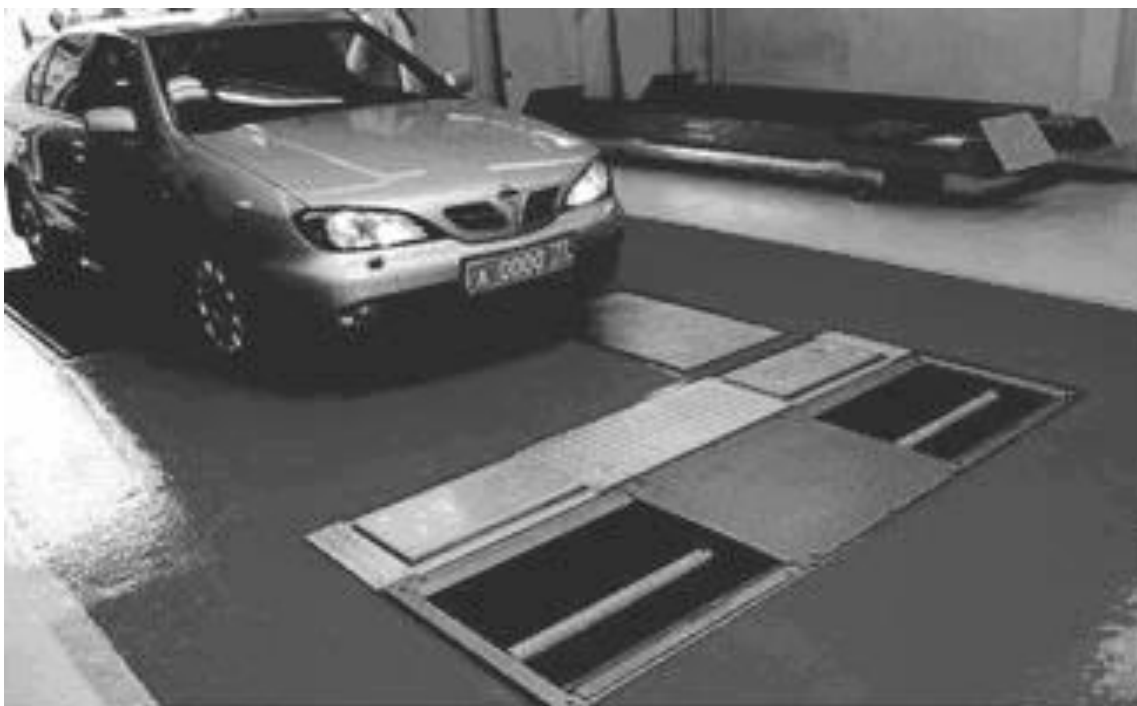
6.24-rasm. LTK-3P-SP-11 rusumli yengil avtomobillar, mikroavtobuslar va kichik yuk avtomobillarini texnik nazorat etuvchi universal diagnostika posti (STS-3P-SP-12 jixozi asosida tayyorlangan, tashqi o'lchamlari 7000x14000 mm).
