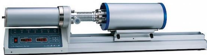
6—rasm. Polimerlanish kinetikasini o'rganishda ishlatiladigan dilatometr.
